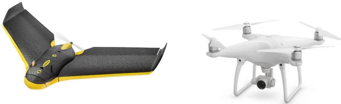
Figure 2. Fixed-wing and Multi-rotor UAVs. Left: eBee senseFly fixed-wing UAV (Source: robots.ieee.org). Right: DJI Phantom 4 multi-rotor UAV (Source: DJI.com).
