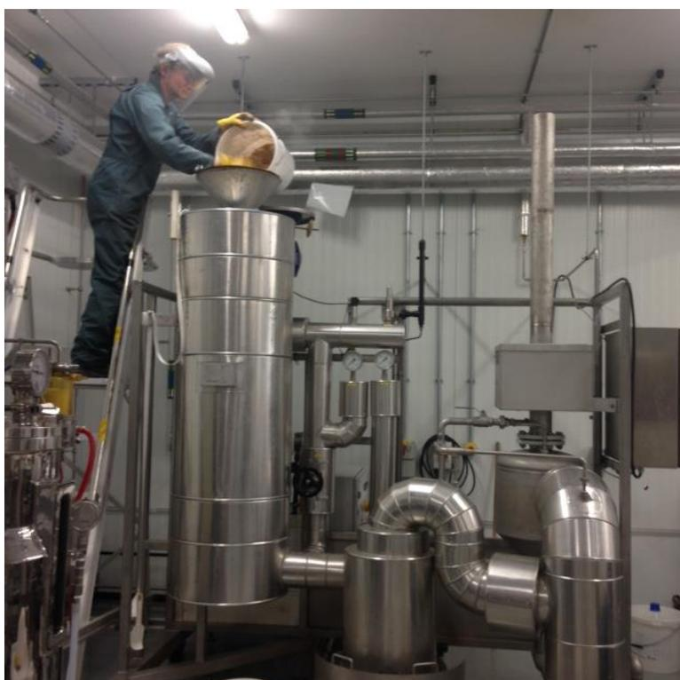
Steam explosion (30L) rig at BEACON biorefining facility
