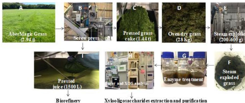
Figure 1: Different steps of the biorefining of grass
