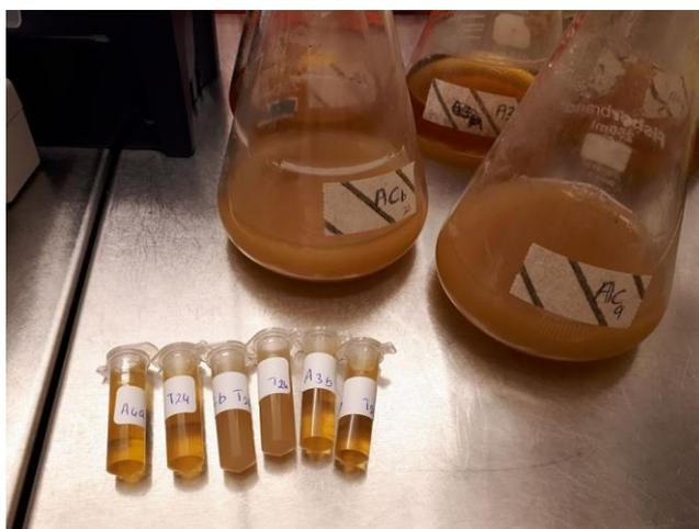
Figure 2: Collected samples of the YEPX medium for HPLC analysis
